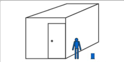
**Fig. 1** Figurative illustration comparing Fanuc's NC system to the US system. A size of a small room is reduced to a mounting on the worktable
